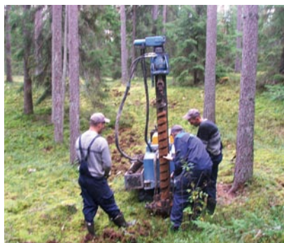
Digging of the sampling well in the forest protective belt
